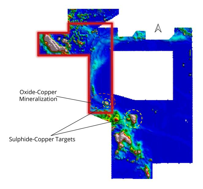
Mitu features several initial sulphide copper targets, including a target which is also associated with a large, known area of nearsurface oxide copper mineralization
